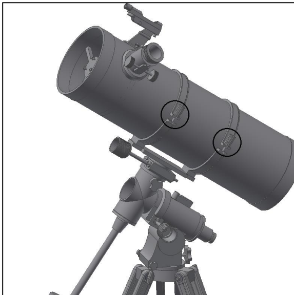
Figure 9. Slide tube and thread the ring knobs.
