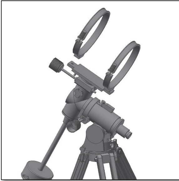
Figure 7. Place the tube rings.
