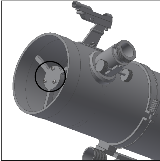
Figure 17. Adjust the secondary mirror.
