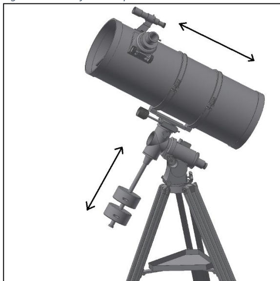
Figure 14. Balance the telescope.
