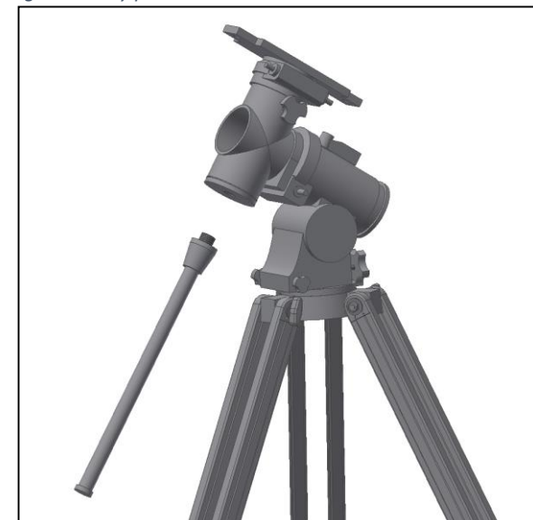
Figure 5. Thread the counterweight shaft.
